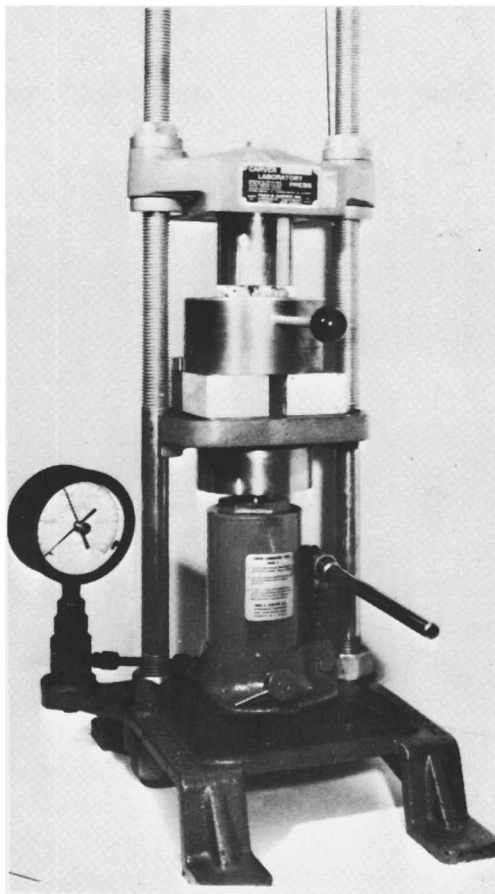
Figure 16. Lyophilized muscle tissue being compressed into an aluminum can. Between 150 and 250 grams of tissue can be compacted for counting
